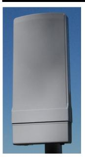
The RapidLink 5525 is a dual radio solution that supports both 2.4 and 5 GHz bands concurrently. The RL-5525 can be configured as dual AP's or one AP and one Backhaul. MESH topologies are supported as well.
