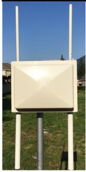
The RapidLink 6725-N-HP is a high power dual radio solution that supports both 2.4 and 5 GHz bands concurrently. The RL-6725 can be configured as dual AP's or one AP and one BackHaul. MESH topologies are supported as well.
