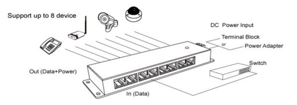
**Overview:** Simple Power of up to 8 Passive Gigabit PoE devices by one power source. Power by DC jack or Terminal Block connector. Applications include wireless access points, IP cameras, IP phones and other POE based devices.
